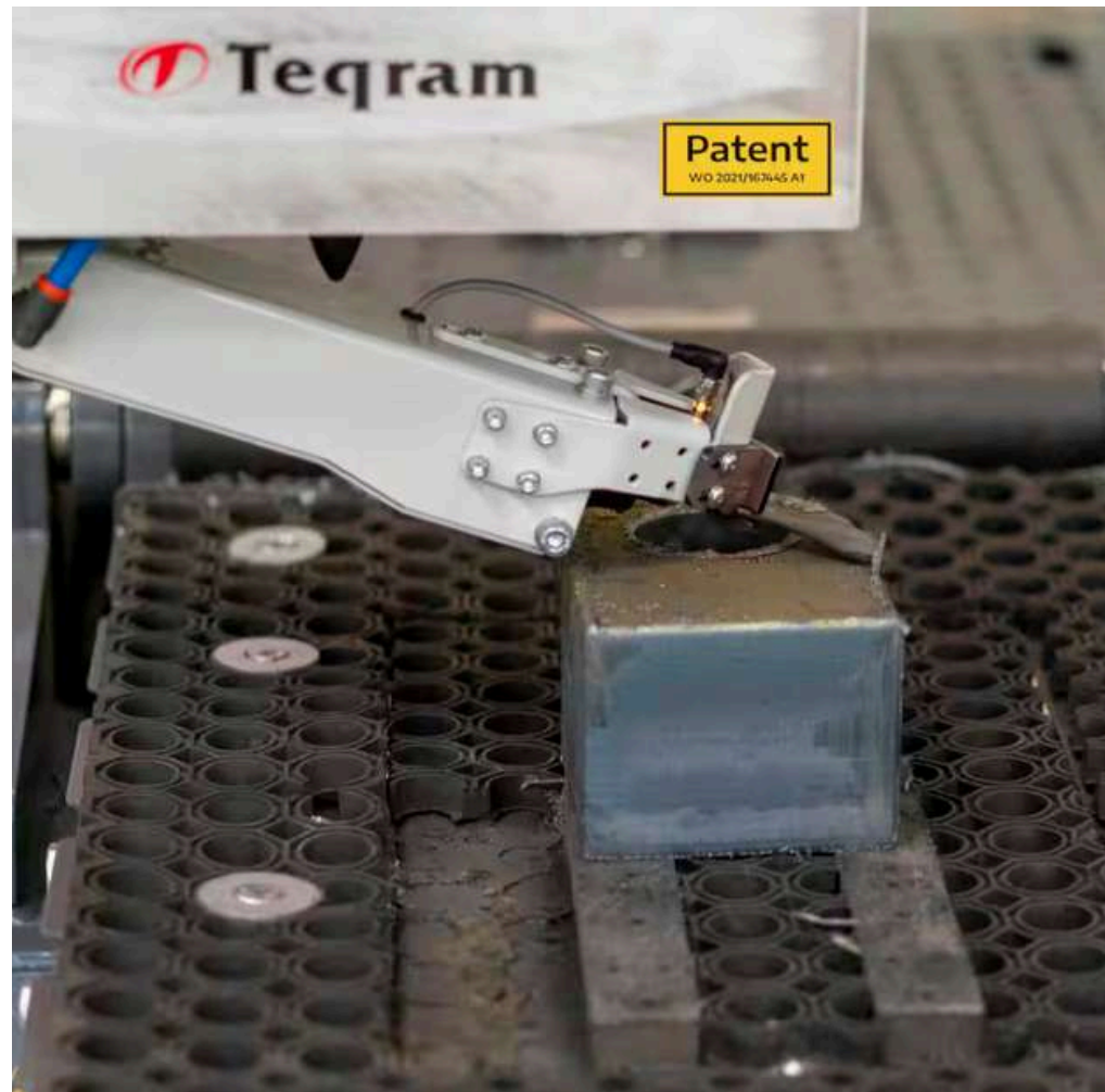
Robotic deslagging with chisel tool
