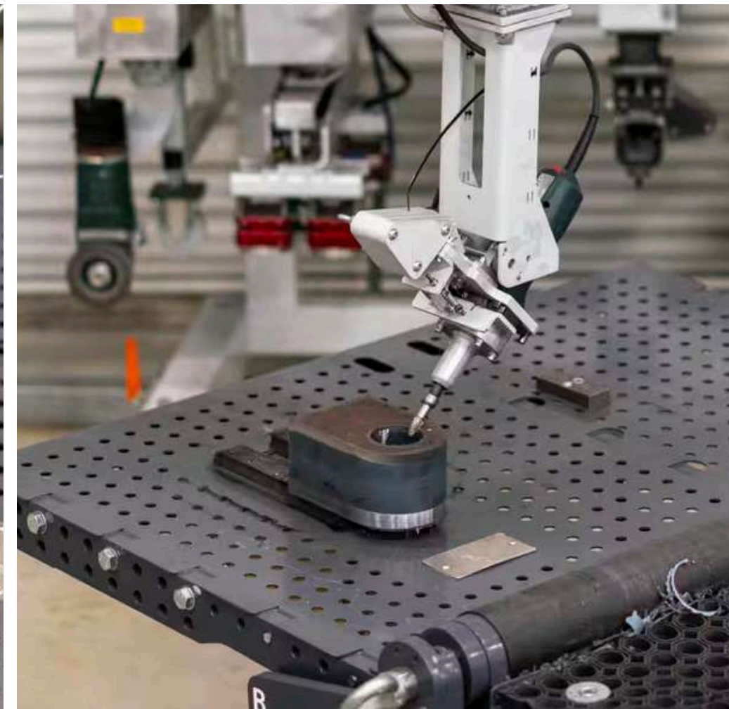
Edge-breaking, edge-rounding and chamfering with die-grinder
