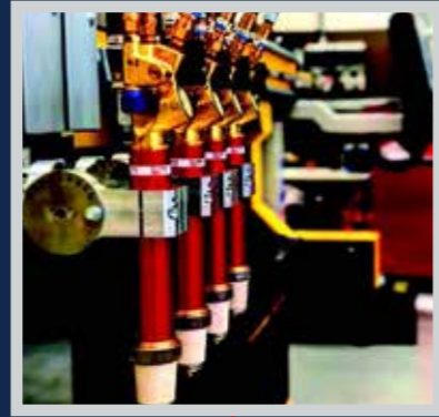
Ossitaglio con capacitivo integrato Flame cutting burner with internal ignition and integrated automatic height control
