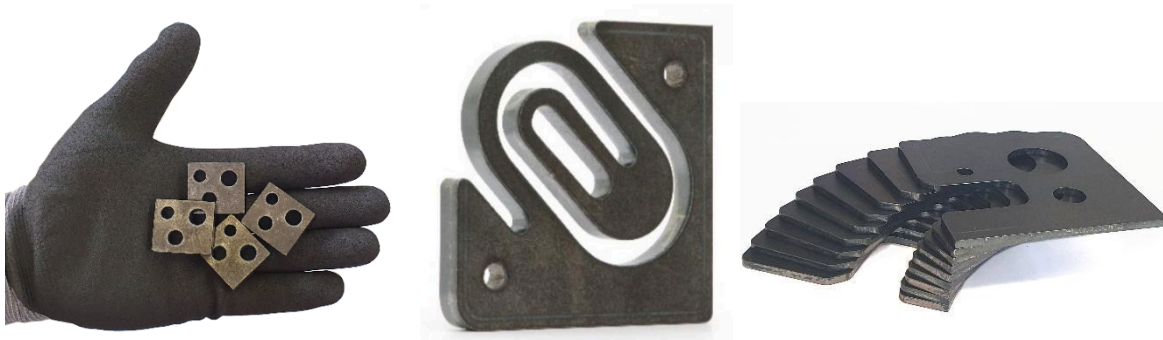
Picture 3: plasma cutting of small holes, narrow webs, and fine contours.
