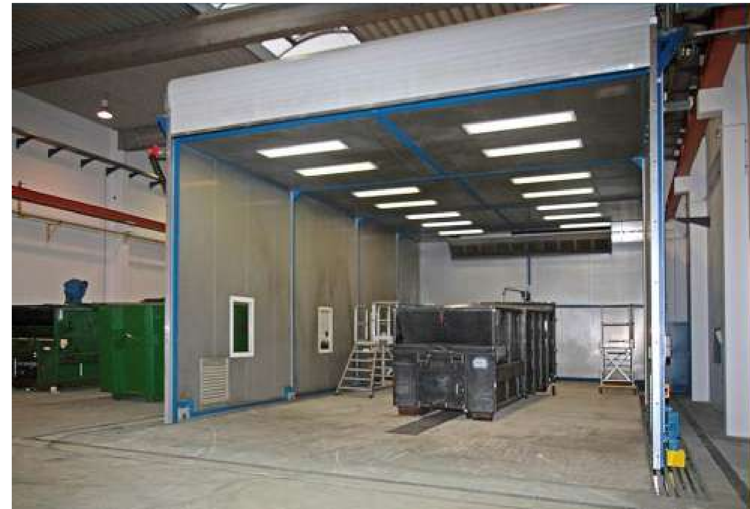
Telescopic high-pressure cleaning booth
