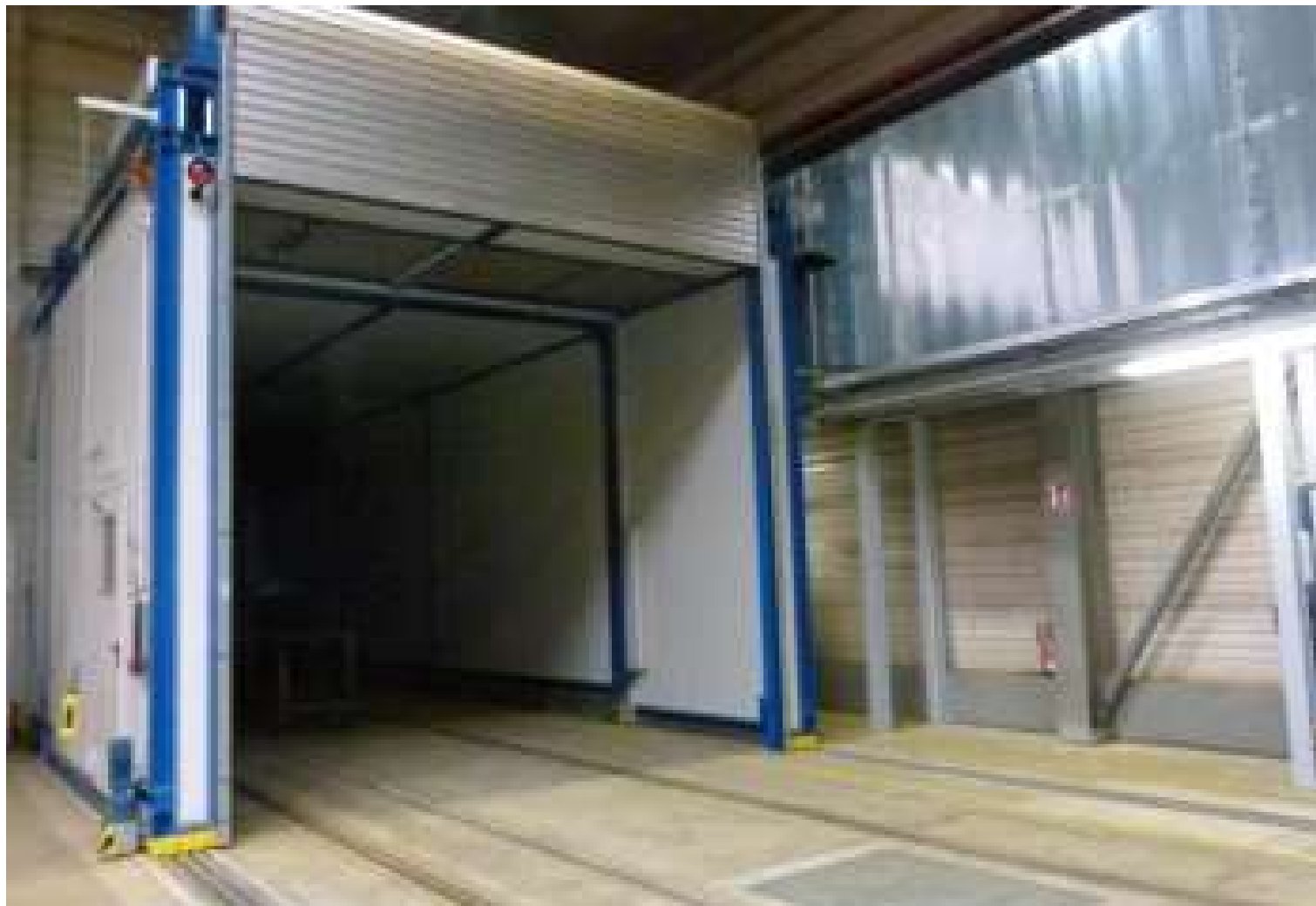
Telescopic dryer retracted
