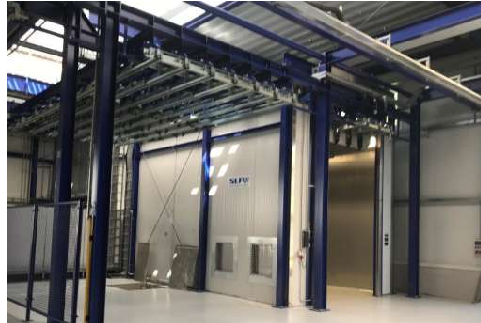
Fully automatic work piece transport
