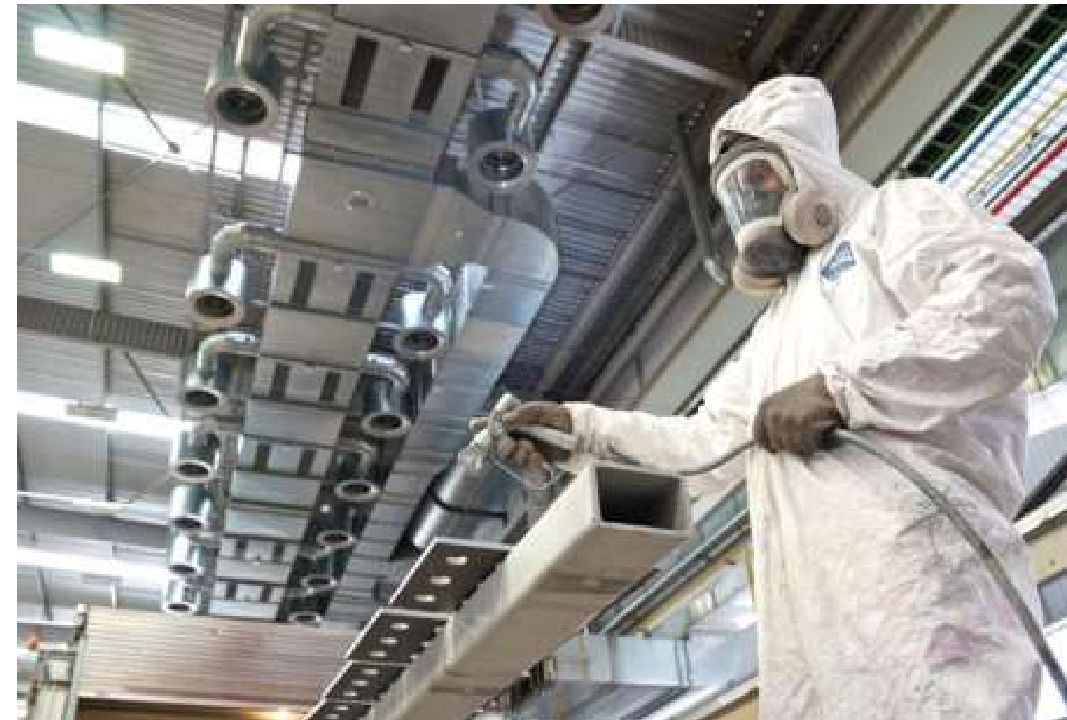
Open-space paint spraying system with telescopic dryer
