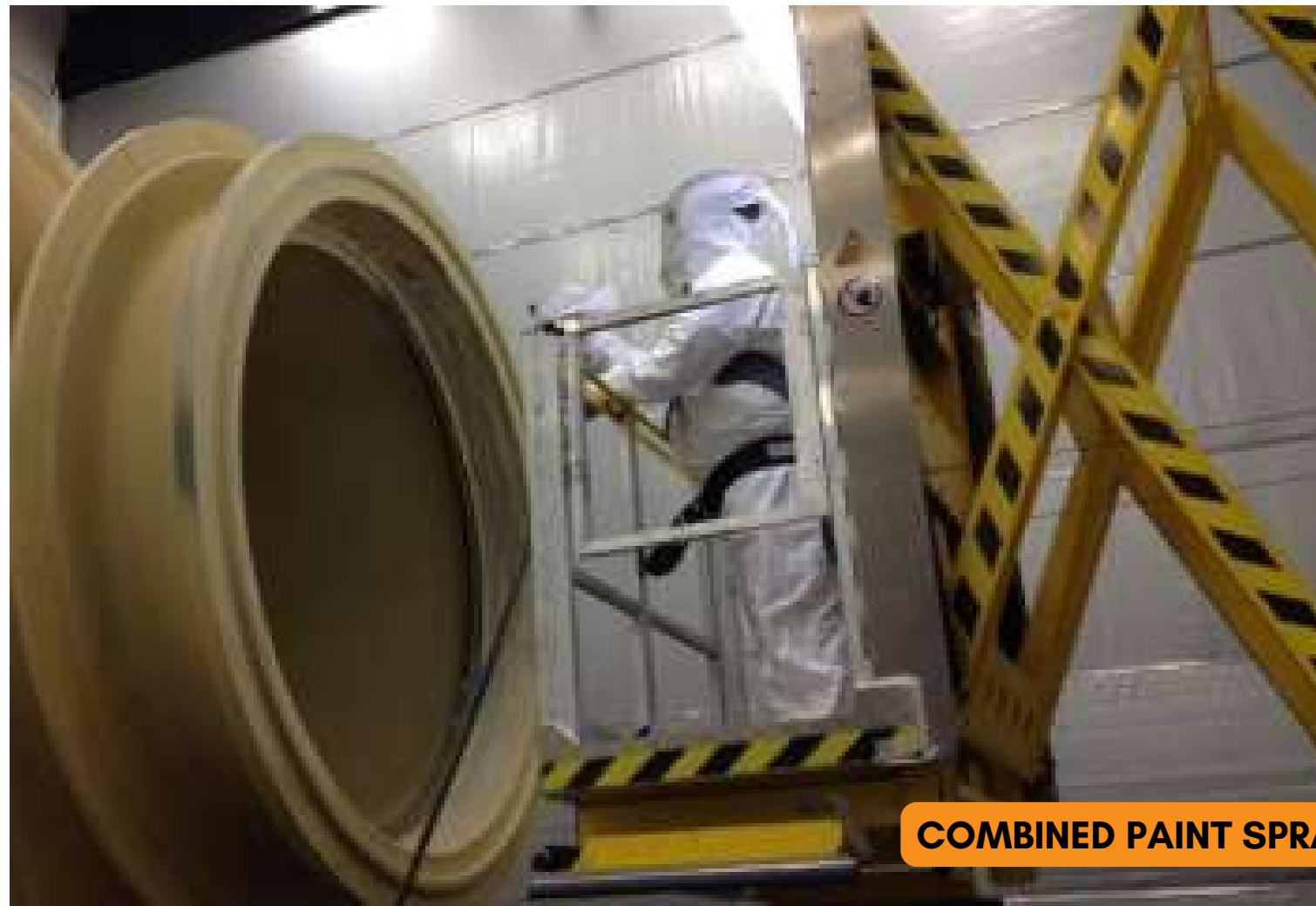
Combined paint spraying and drying booth with horizontal scissor-type lifting platforms
