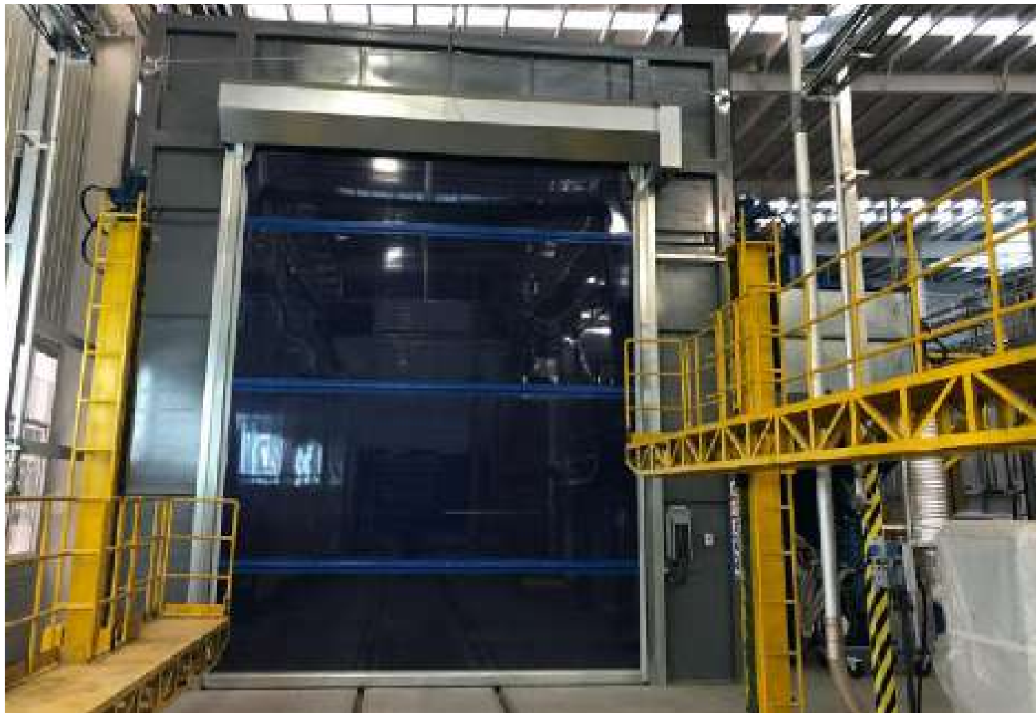
Sandblasting room with two electrically operated roller doors on the frontal sides
