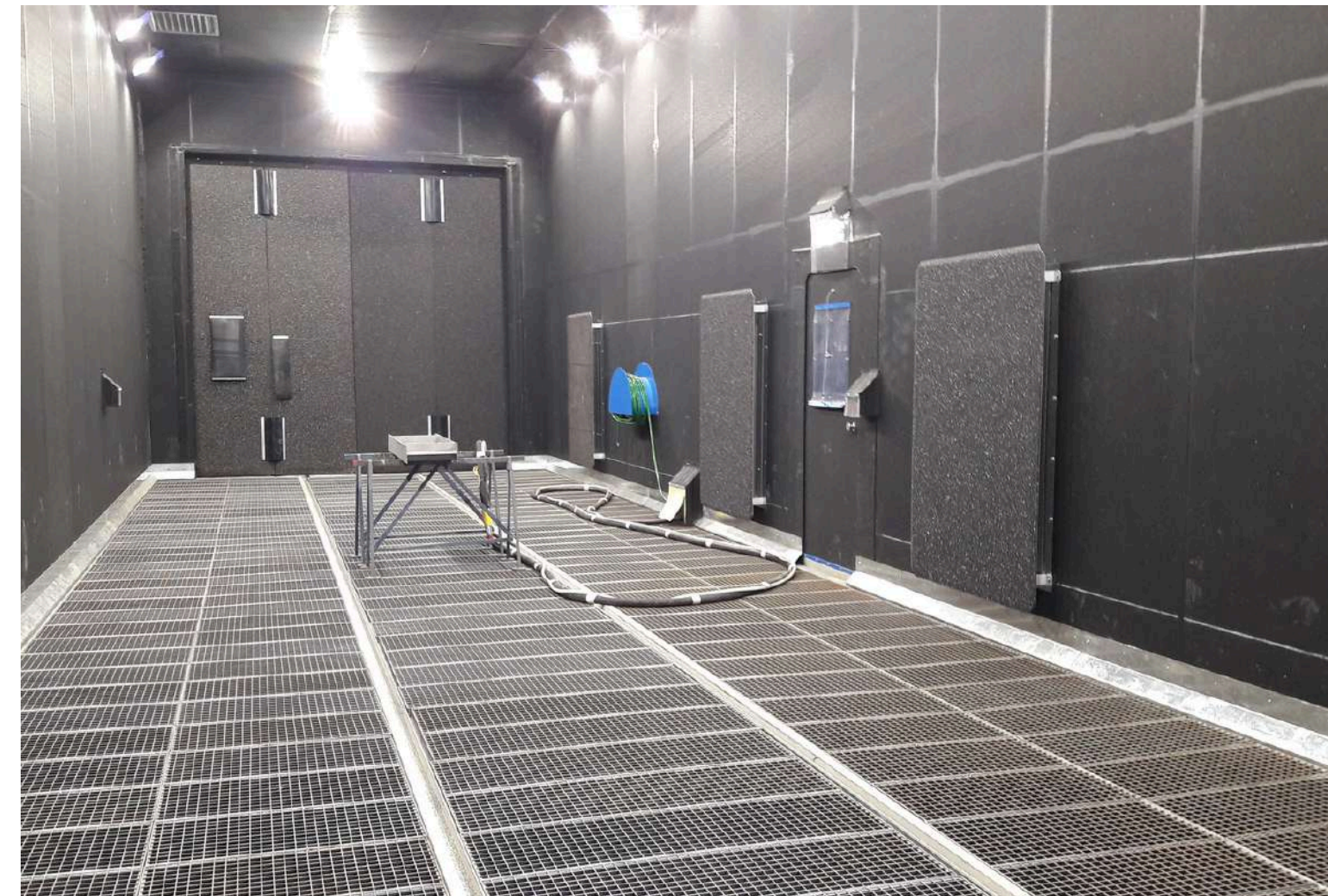
Interior view of the blastroom with floor completely covered with gratings
