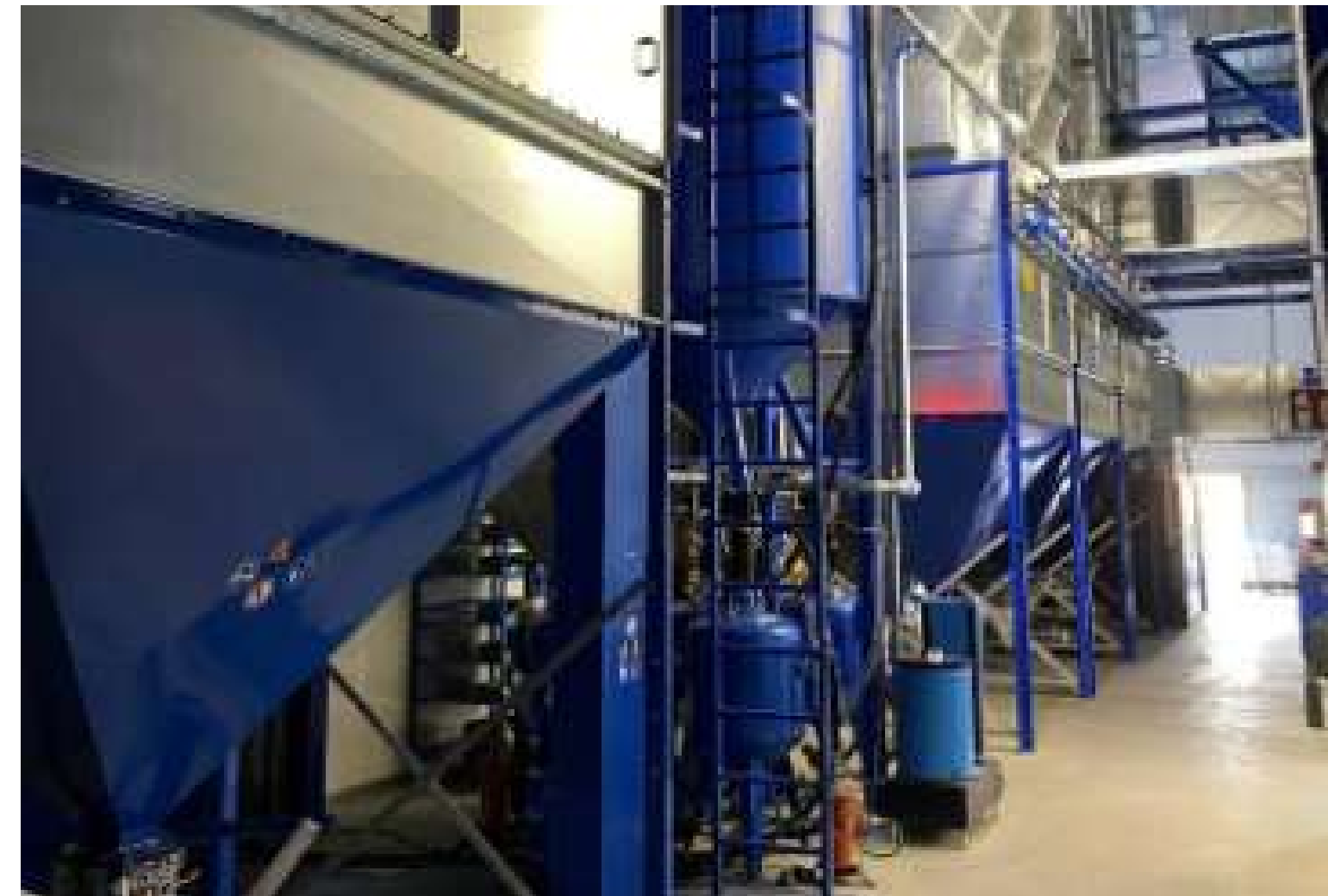
6 filter systems with suction power of 105.000 m 3 /h
