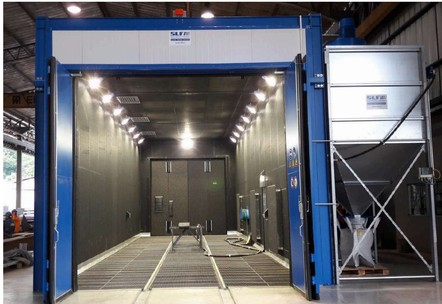
Interior view of the blastroom with floor completely covered with gratings
