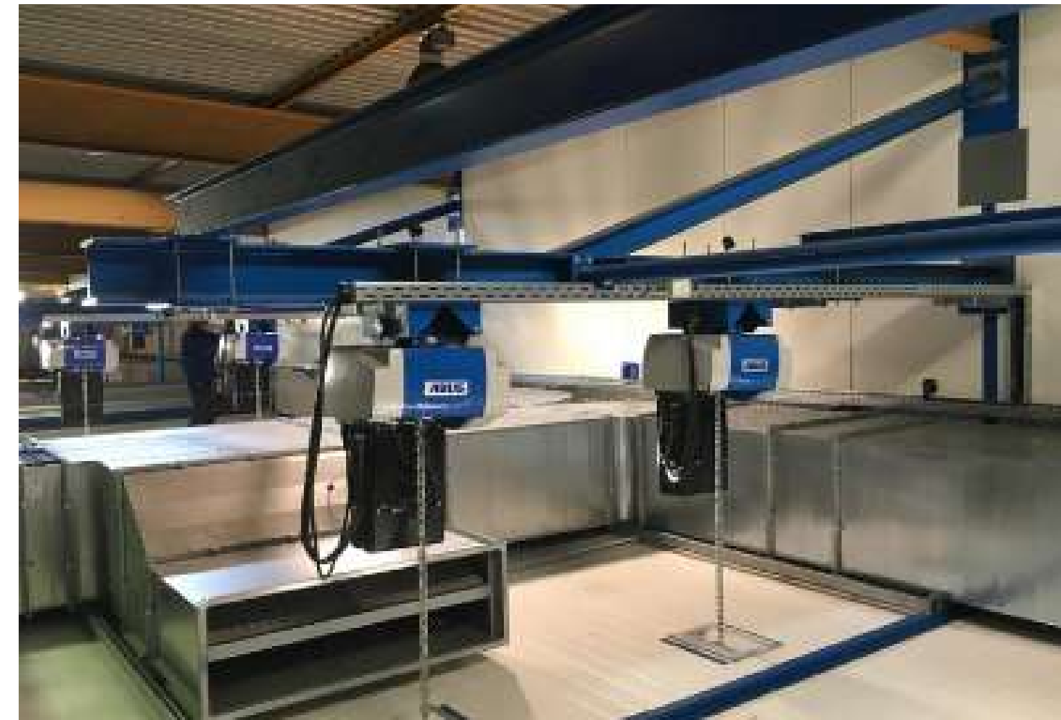
Sandblasting room with chain hoists for suspending the parts to be treated
