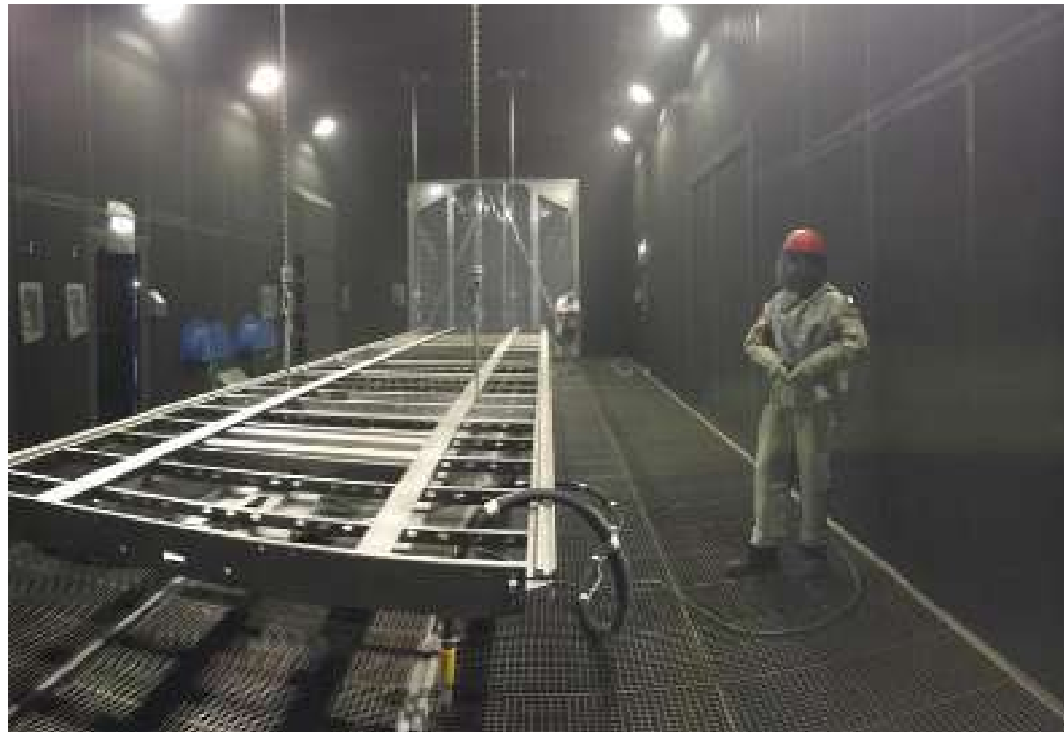
Sandblasting room with chain hoists for suspending the parts to be treated
