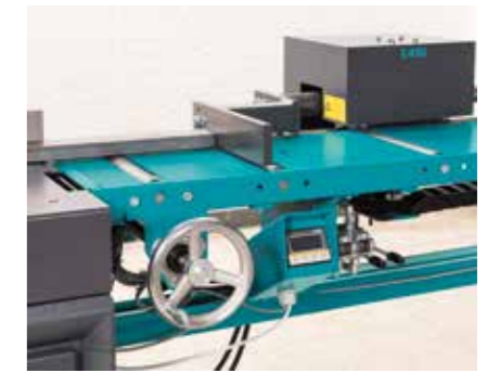
L 45 I length measurement device The stop is moved using a handwheel; the clamp is operated hydraulically by a hand valve. Digital length display.
