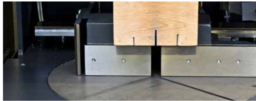
Rotary table for mitre cuts with a pivoting range of 180°.
