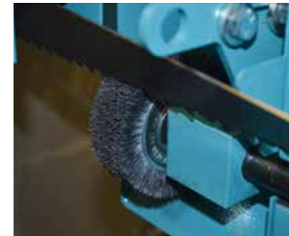
Independently driven swarf brush.
