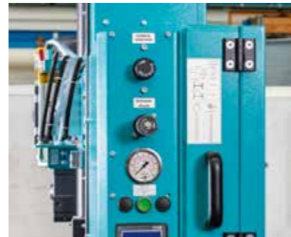
Hydraulic saw band feed, steplessly adjustable.
