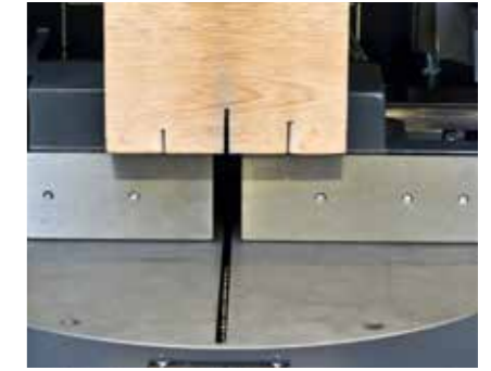
Vertical hardwood clamping block to protect material surface.
