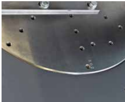
Drilling pattern in the saw table for clamping fixtures of the customers own design.
