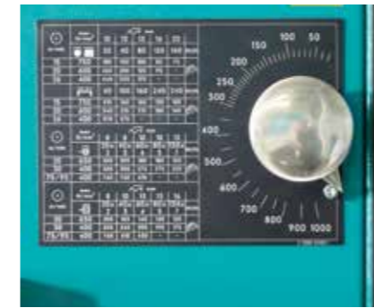
Hydraulic saw blade feed, infinitely variable according to table.
