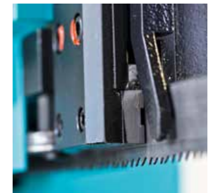
Carbide-tipped saw band guides of the KBS series.
