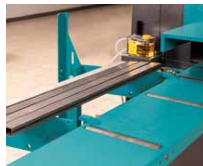
Material rest For temporary storing of cut material (optional).
