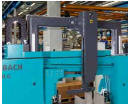
Saw frame pre-stressed running on play free linear bearings.
