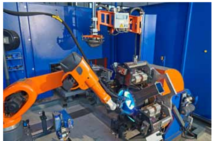
Welding of the interior cover seams with best accessibility due to the 90° special torch at the QRC 320 robot
