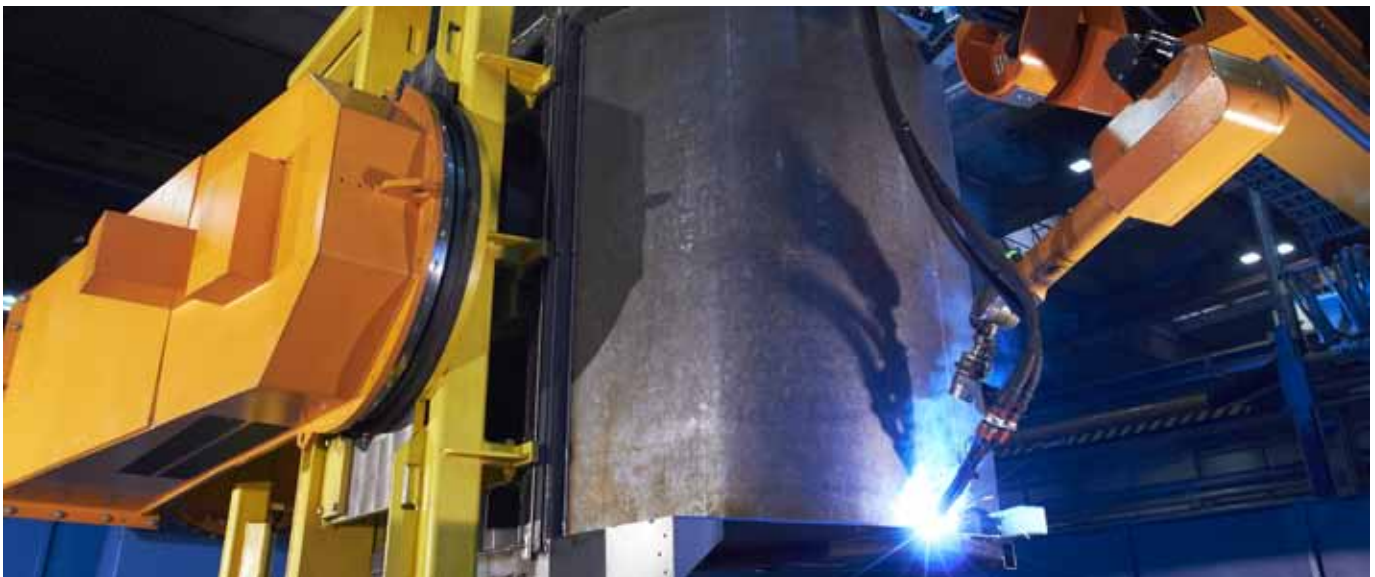
The different container types are welded in 4 stations which can be operated independently from each other. The completed container meets the highest standards of tensile strength and weld quality and allows an optimum waste compaction.
