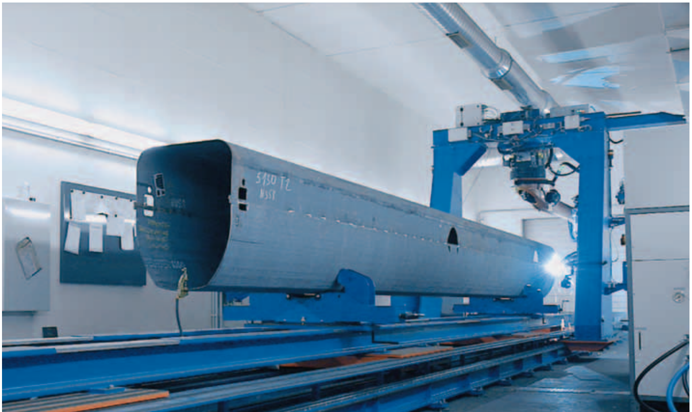
The boom of a mobile crane comprises a main element and up to 6 six telescopic sections, each of which can measure up to 14 m. The lower half is made of a thicker plate than the upper half. High-strength fine-graded steels with material thicknesses from 4 to 15 mm are used to produce the boom sections.
