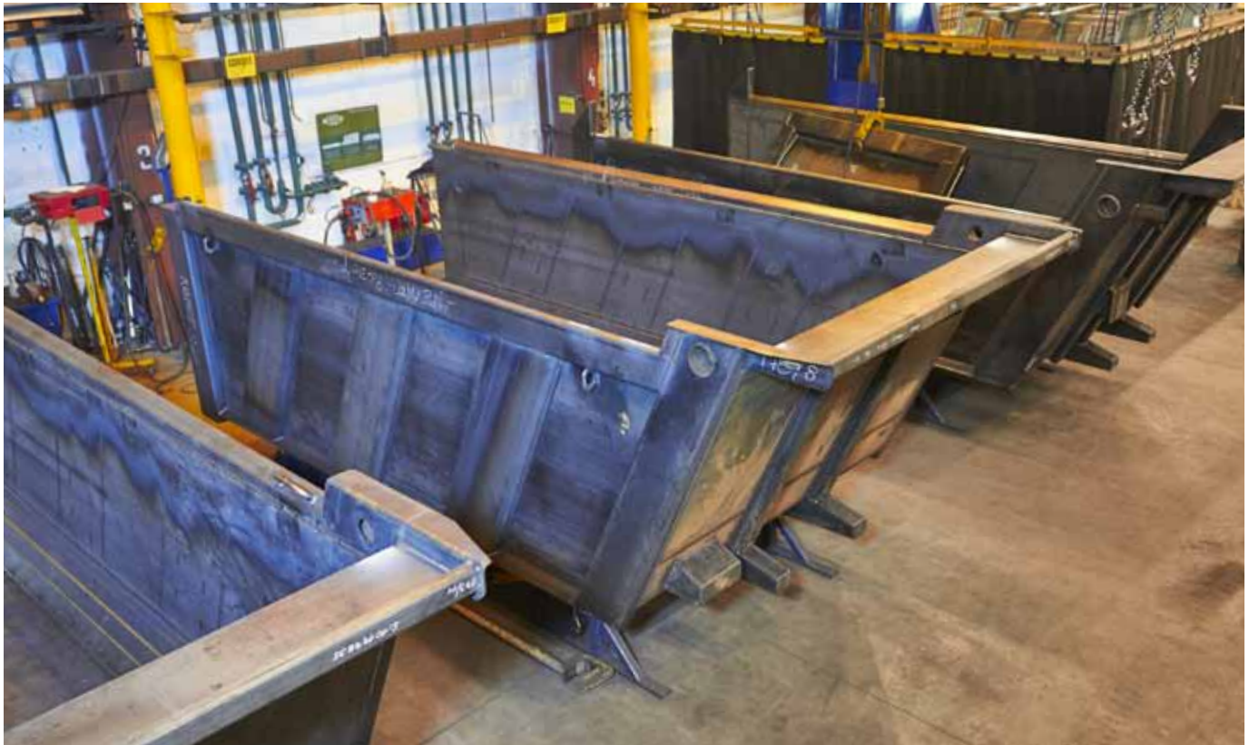
At the Slaný site the tipper bodies for rear tippers, three-way and two-way tippers are produced and later exported to Europe and Asia.
