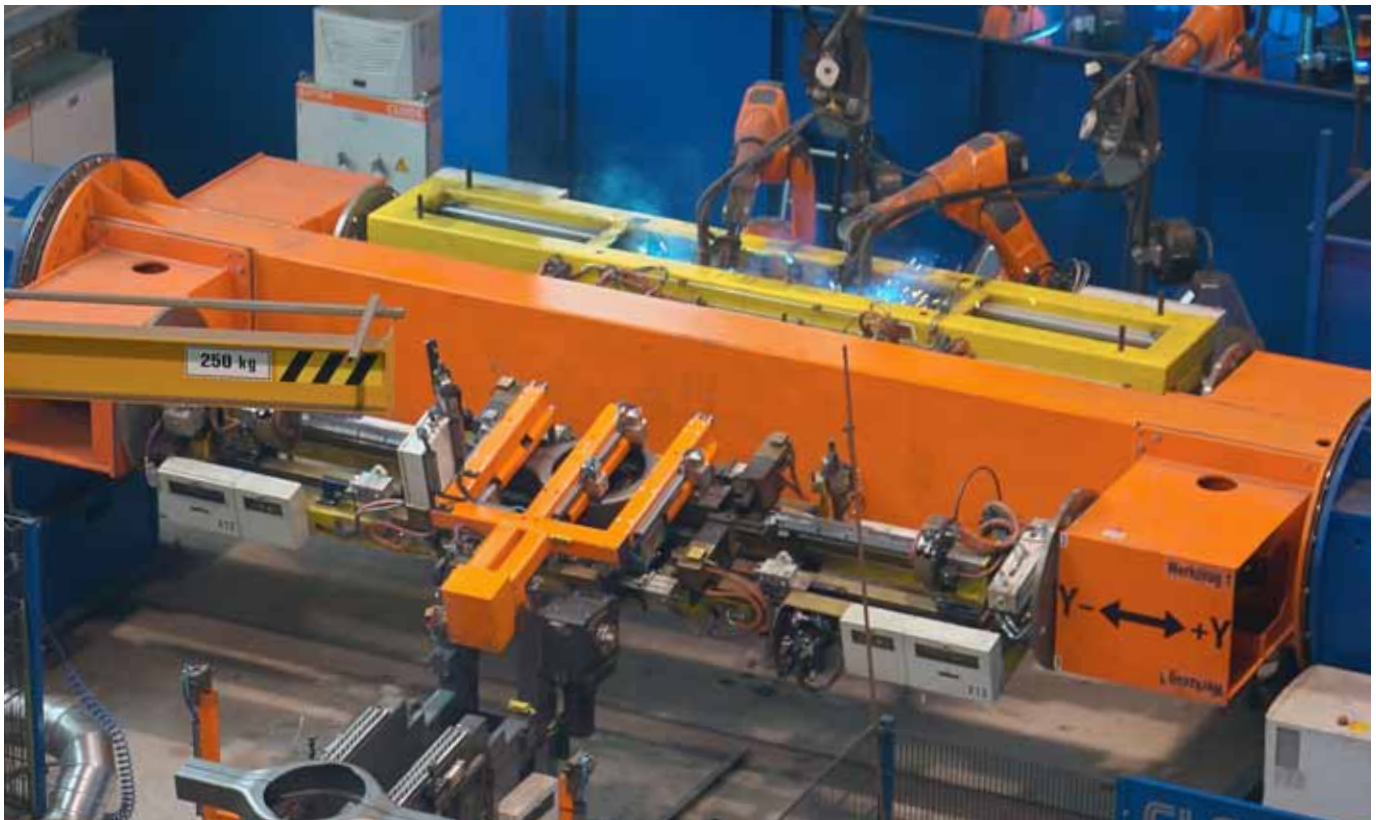
The system comprises a total of six stations which are operated by only two workers. The output quantity in 3-shift operation is 75,000 axles. The stations are chained, the components are loaded via a shuttle system.
