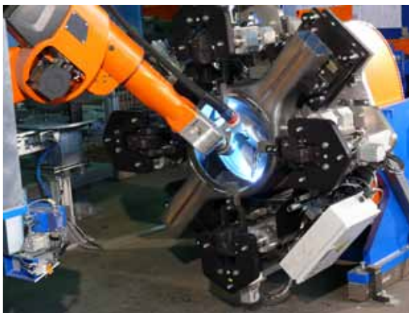
Measurement of the axle casing by means of a laser offline sensor and then root pass welding to both sides
