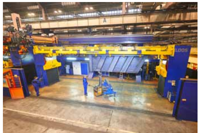
The system comprises three workstations which are arranged in a line. Thus the processing time during production is reduced considerably.
