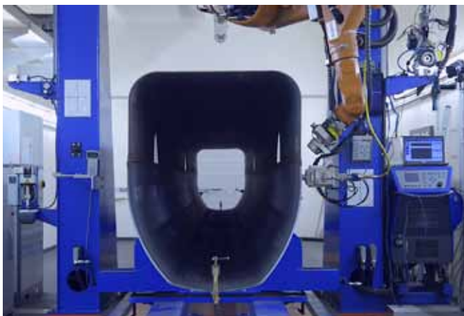
The automatic position marking for the holes is now made 80 % faster compared to manual cutting.
