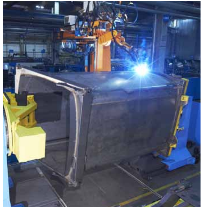
The container is 3 mm thick and Tandem welded.
