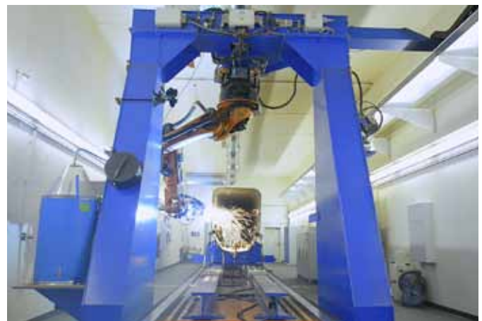
By hand, each hole took 15 min. The laser produces up to 30 holes in the same time.
