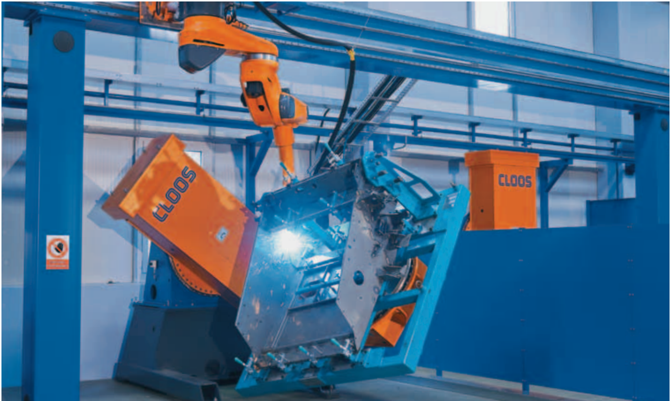
The overhead-mounted CLOOS 7-axis QRC-E 350 robot welds the combine frames with optimum accessibility
