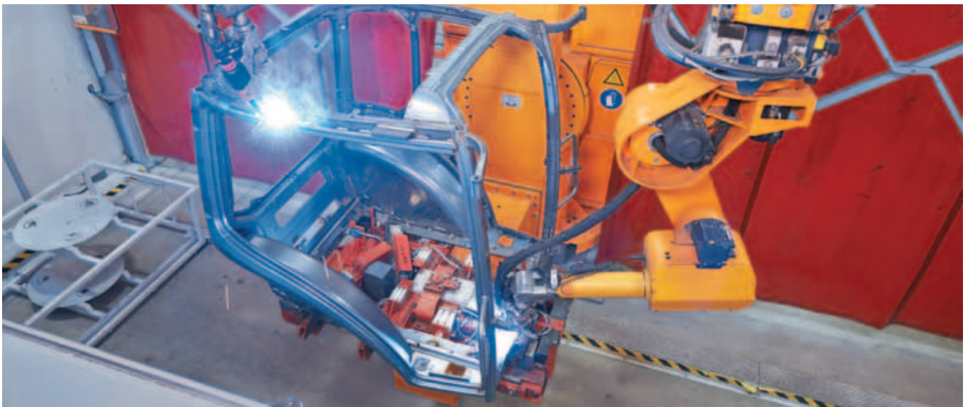
The different cab variants can be welded without conversions or set-up changes
