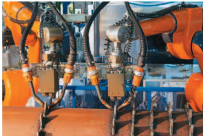
Two QRC 350-type robots automatically collect the fork arms as bulk material and locate them optimally on the component
