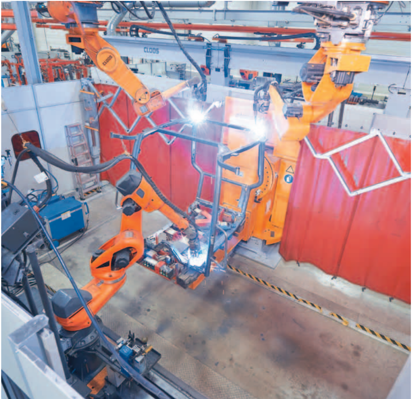
Three QRC-E 350- and QRC 350-type QIROX robots weld the different cab variants
