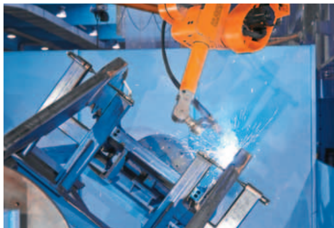
Positioning of the component in the optimum welding position
