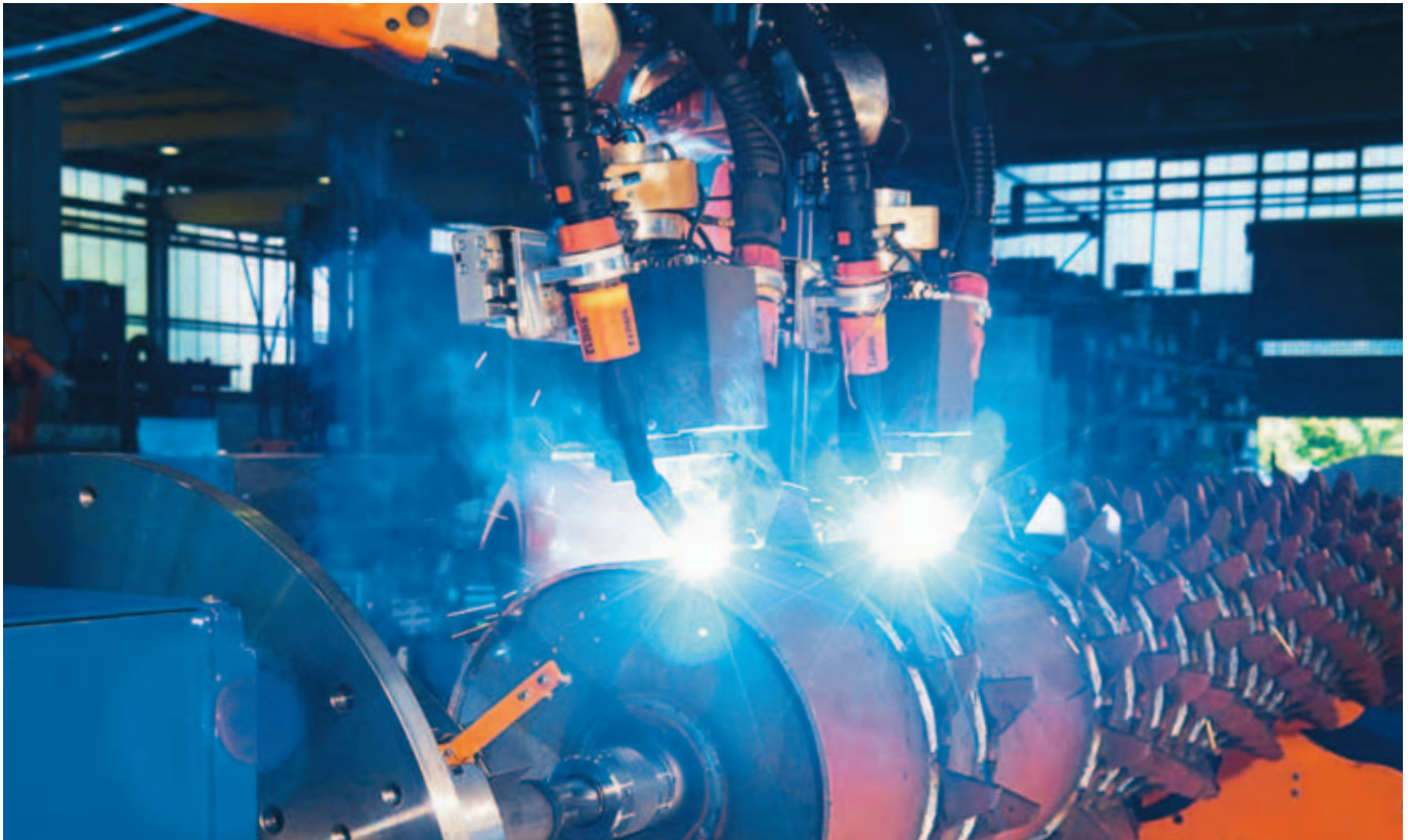
The welding torches with gripping system locate the fork arms on the roller and carry out welding
