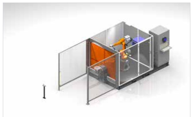
QIROX Compact cell QR-CC-6.1 with 2-station positioner
