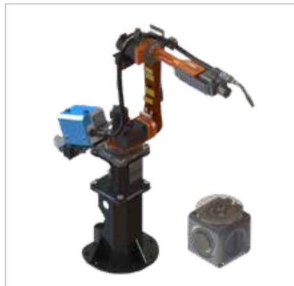
Example 2: QRC-290 with rotary positioner with faceplate in horizontal position
