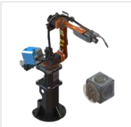
Example 1: QRC-290 with rotary positioner with faceplate in vertical position
