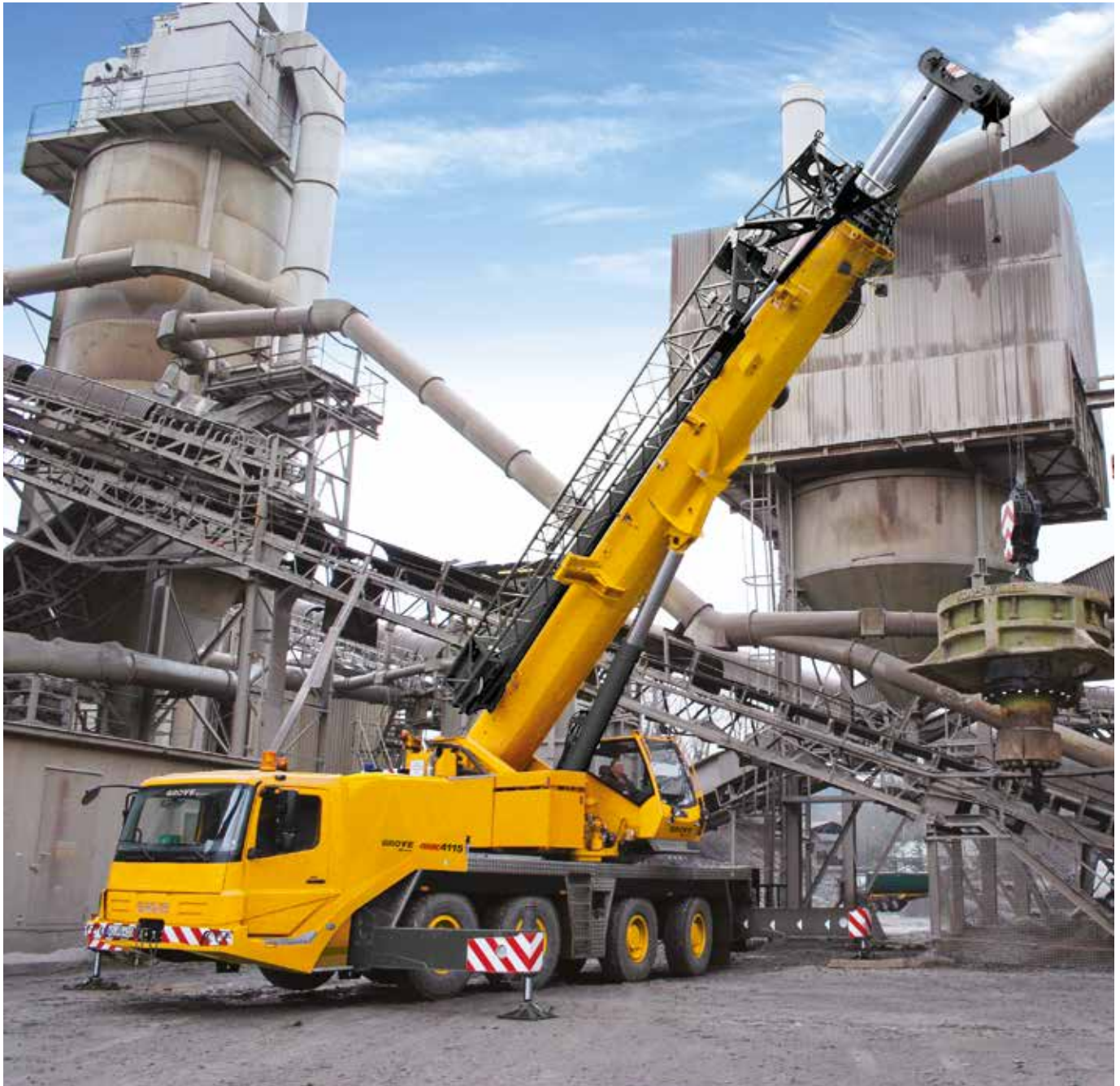
The Grove GMK4115 mobile telescoping crane with a max. capacity of 100 t, 11.3 m boom length and a boom angle of -1.5^{\circ} to max. +82^{\circ} .
