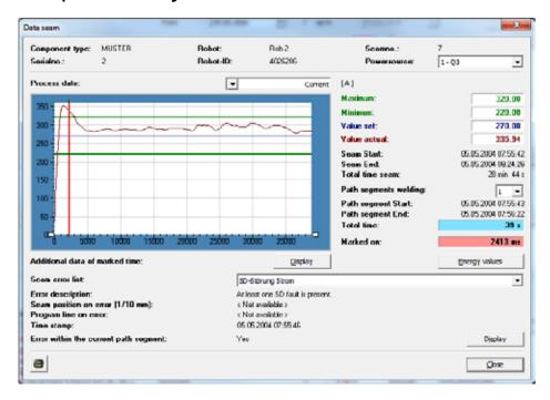
The process data of every recorded weld seam can be shown as graphics,.
