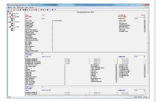
Robot operating data and process data of the power sources can be visualised online.
