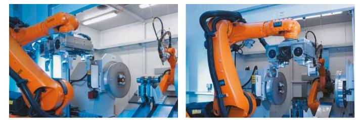
For the commercial vehicle sector CLOOS realised a turnkey laser MIG/MAG production line. Hydraulics jacks for tipper bodies and trailers are welded on the system. Thus the laser MIG/MAG technology achieved the breakthrough also when welding thicker plates.
