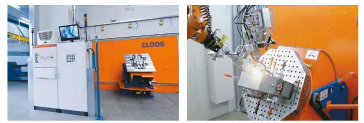
The Luxemburg company TMS Metall- und Stahlbau wants to capture new markets and so is investing in a state-ofthe-art laser welding system with robot technology from CLOOS. For the first time a Scan-Tracker optic is used for heat conduction welding so that different materials and weld geometries can be reliably processed.
