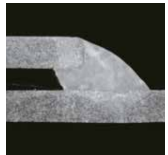
Overlap weld with gap
