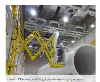
respective requirements, we design our lifting platforms to be particularly wear- and dust-proof for use in blastrooms and in a splashwater protected or explosion-proof design for use in potentially explosive areas such as paint-spraying booths.
