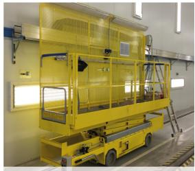
Mobile, movable lifting platform in paint-spraying booth
