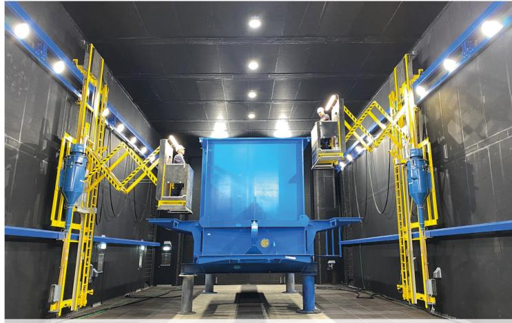
The **SLF** scissor-type lifting platforms enable a continuous and complete blast cleaning process from the work platforms, even with very large workpieces.
