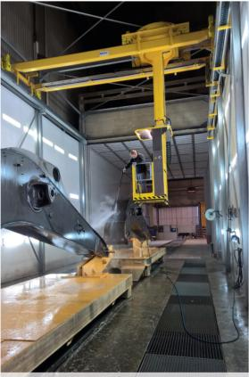
Vertical telescopic lifting platform with turnable work platform (+/- 180°)
