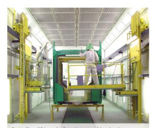
Swivelling lifting platform in a combined paintspraying and drying booth
