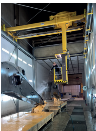
SLF blastroom with blast media robot ReCo-Blaster®, crane bridge-guided in rotating device.
