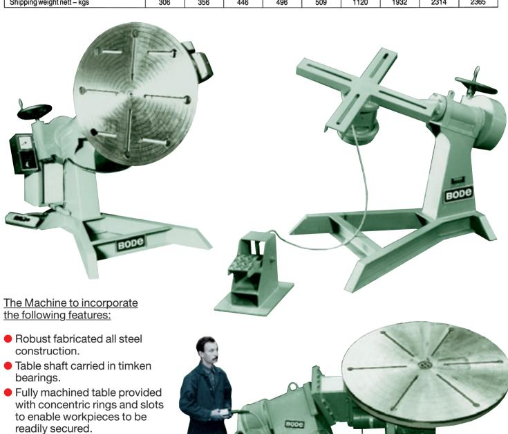
Self-locking worm gear tilt drive.
