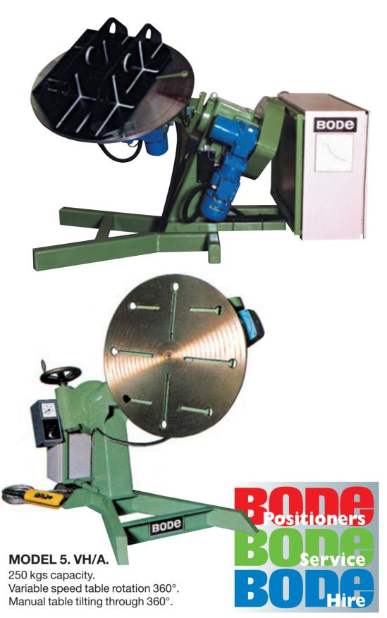
Machine equipped with a diameter selector enabling the operator to set the table rotation speed required for the workpiece diameter
