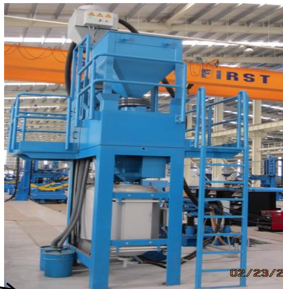
Flux recovery and recycling system
