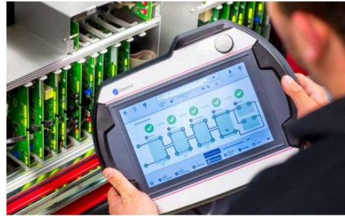
Mobile control unit, freely positionable
