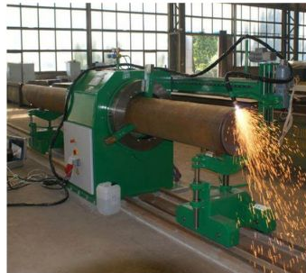
PIPE ROTATORS AND PIPE WELDING
