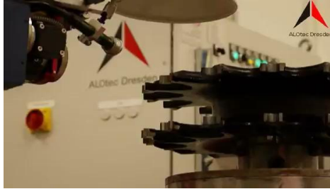
LASER HARDENING OF A SPROCKET
