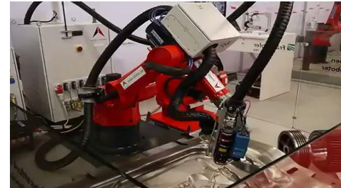
LASER HARDENING OF A FORMING TOOL
