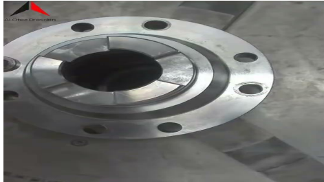
LASER HARDENING OF A COUPLING PIECE
