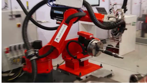
LASER HARDENING OF TRANSMISSION COMPONENTS
