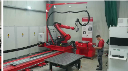
STATIONARY LASER SYSTEM WITH TURN-TILT AXIS
