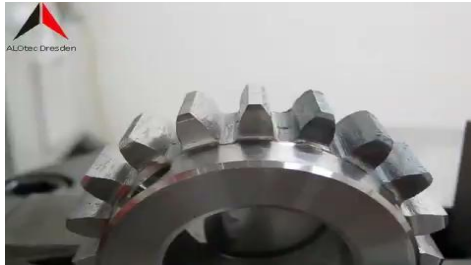
LASER HARDENING OF A GEAR
