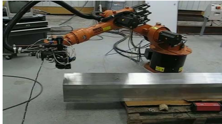
LASER WELDING WITH SPOT-IN-SPOT DESIGN
