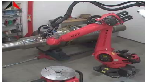
LASER POWDER DEPOSITION WELDING ON A ROLLER
