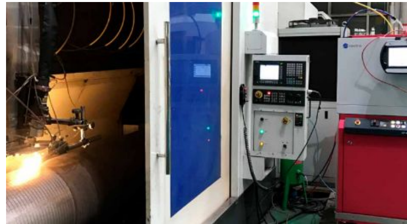
Here a 10 kW laser for cladding of mine cylinders in a machine of Anyang Rui Heng CNC Machine Tool Co., Ltd., Anyang City / China.
