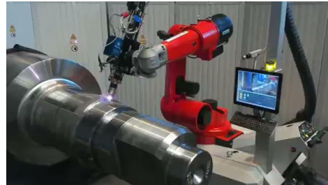
LASER POWDER DEPOSITION WELDING OF A ROLLER
