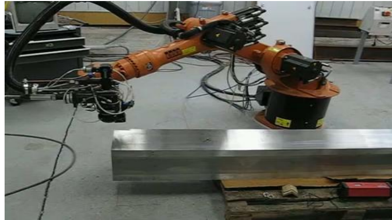
LASER WELDING WITH SPOT-IN-SPOT DESIGN
