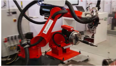
LASER HARDENING OF TRANSMISSION COMPONENTS
