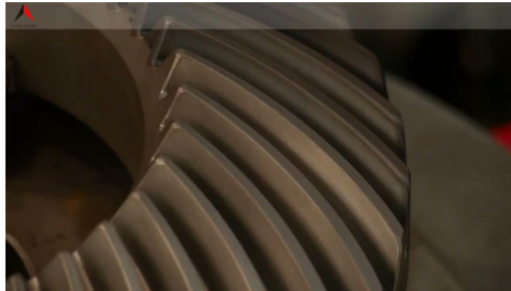
LASER HARDENING OF A BEVEL GEAR
