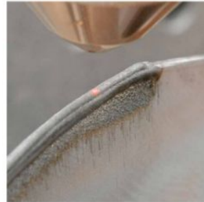
Wear protection of saw-blades, disc harrows or counter blades in agriculture and forestry.
