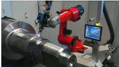
LASER POWDER DEPOSITION WELDING OF A ROLLER
