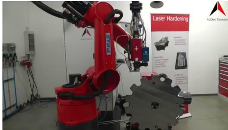
LASER HARDENING OF A GEAR - 7 ROBOT AXES SIMULTANEOUSLY
